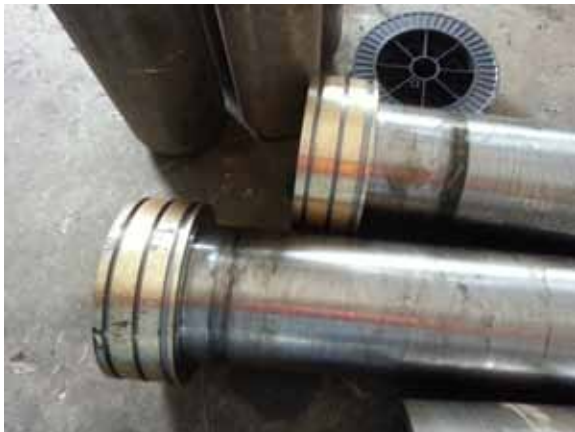
Scenes of Production (Copper Plated Piston for Stressing Jack)
